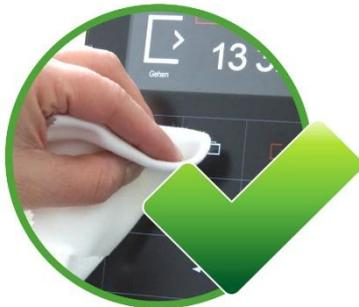
Never use scouring milk or caustic cleaning agents to remove dirt. Especially the displays as well as the keyboard and fingerprint modules must be cleaned carefully.
